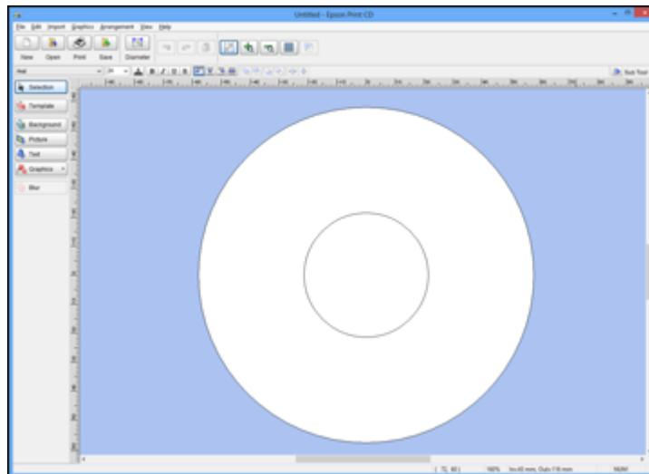
2. Use the buttons on the left side of the screen to select a pre-designed template or add a background image, picture, text, or graphic elements. For more information, select the **Help** menu.
