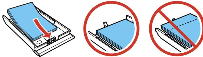
**Note:** Make sure the paper is loaded against the front edge guide and not sticking out from the end of the cassette.
