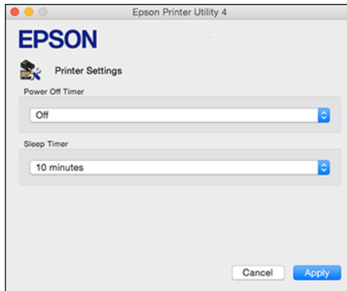
4. Select the length of time after which you want the product to automatically turn off when it is not in use as the **Power Off Timer** setting.
