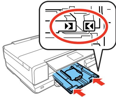
**Note:** The output tray opens automatically when you print. Leave enough space in front of the product for the paper to be fully ejected. Do not remove or insert the paper cassette while the product is operating.
