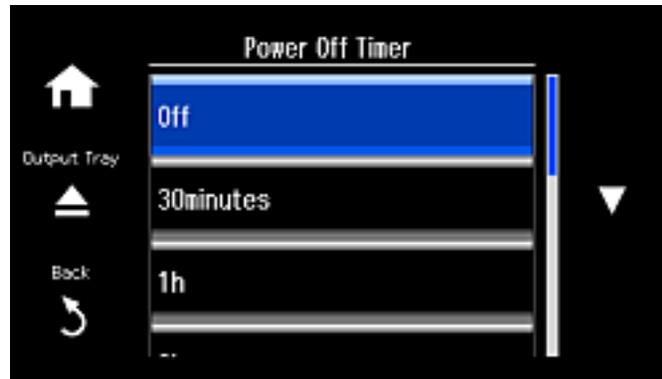
5. Press the up or down arrow button to select the length of time after which you want the product to automatically turn off when it is not in use.
