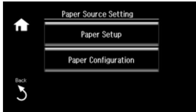
**Note:** To turn off the automatic display of the paper settings selection screen after paper is loaded in the cassettes, set the **Paper Configuration** setting to **Off**. If you do this, you will not be able to use AirPrint.
