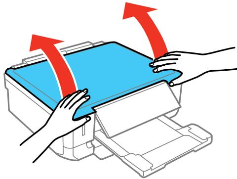
2. Place your original facedown on the scanner glass with the top of the original facing into the corner shown. Slide the original to the edges of the indicated corner.
