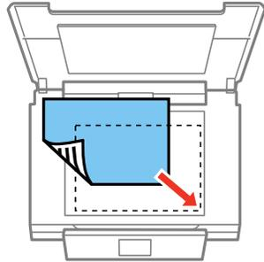
**Note:** You can place multiple originals on the scanner glass. Just make sure they are at least 0.20 inch (5 mm) away from each other and from the edge of the scanner glass.
