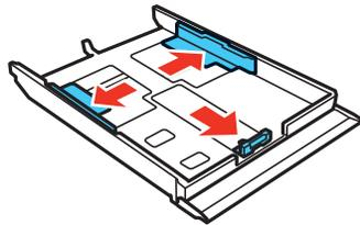
**Note:** If you are using legal-size paper, remove the CD/DVD tray from under the lower cassette. Press the button on the lower cassette and extend it as shown.
