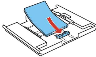
**Note:** Make sure the paper is loaded against the front edge guide and not sticking out from the end of the cassette.
