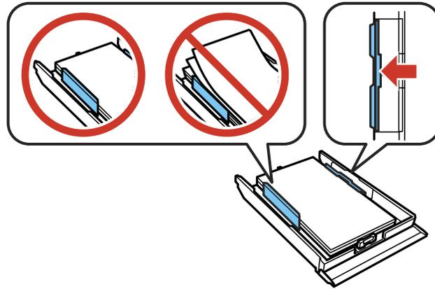
**Note:** Make sure the paper is under the tabs on the edge guides.
