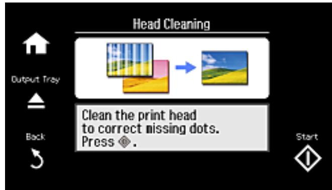
7. Press the **Start** button to clean the print head. You see a message on the LCD screen during the cleaning cycle.
