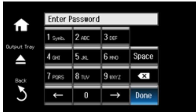
**Note:** The network name and password are case sensitive. Be sure to correctly enter uppercase and lowercase letters, and numeric or special characters.
