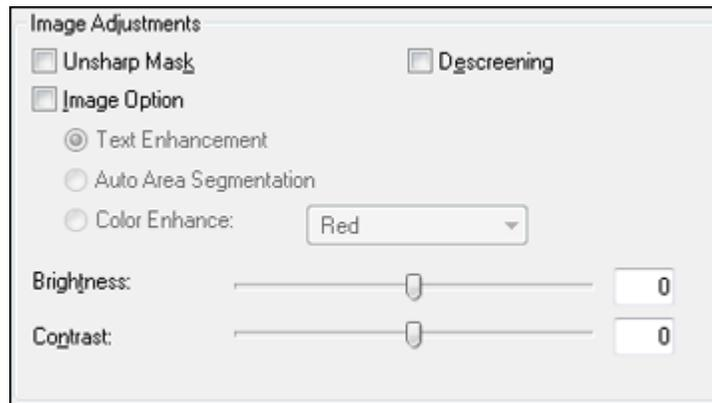
**Note:** Select the **Image Option** checkbox if you need to set any of the grayed-out image adjustments beneath the checkbox. Not all adjustment settings may be available, depending on the Image Type setting.
