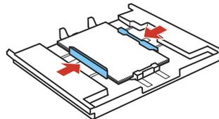
**Note:** Make sure the paper is under the tabs on the edge guides.
