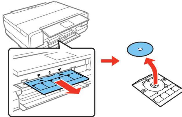
7. Place a CD or DVD on the CD/DVD tray with the printable side faceup, and insert the tray into the slot above the output tray.
