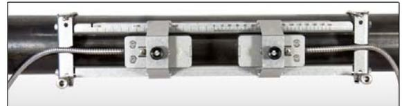
Measurement with transducers mounted by the portable Variofix VP
