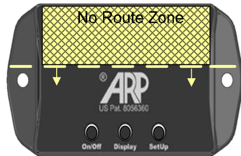
Fig. 6 Housing Wire Routing & Water Drain
