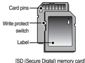
The SD / SDHC memory card has a write protect switch that prevents image files from being deleted or formatted. By sliding the switch to the bottom of the SD memory card, the data will be protected. By sliding the switch to the top of the SD memory card, the data protection will be cancelled. Slide the switch to the top of the SD memory card before taking a picture.
