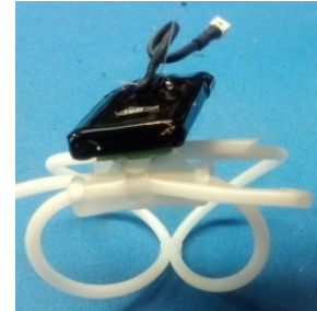
Rat Saddle Harness with Mounted 500 mAh External Battery
