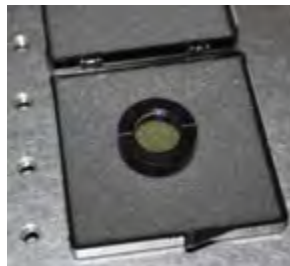
Figure 1.5 – A quarter waveplate retarder.
