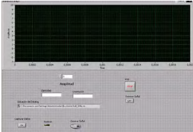
Figure 4.1 – Labview program for controlling the input square signal used to characterise the LCVR
