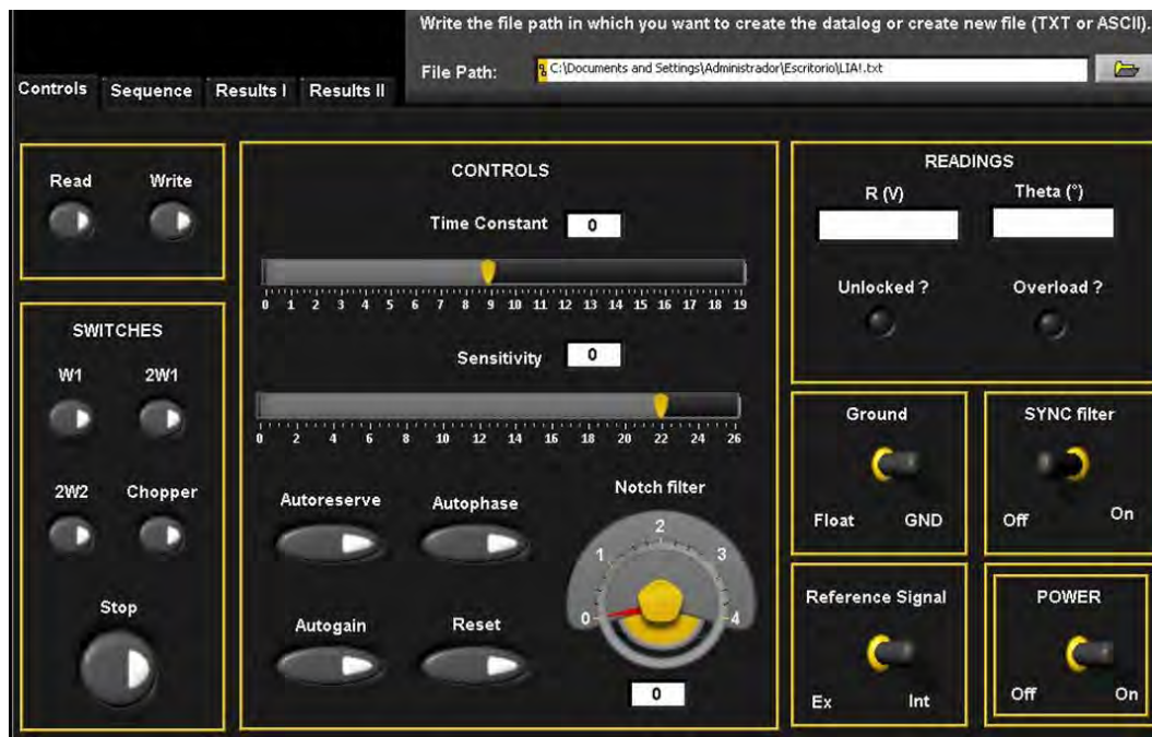
Figure 3.18 – Control panel for manual operation of system
