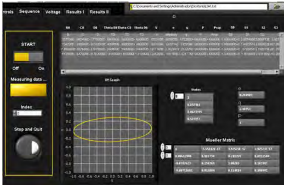
Figure 3.22 – Automatic measurement user panel, displaying the Mueller matrix of the sample under study.
