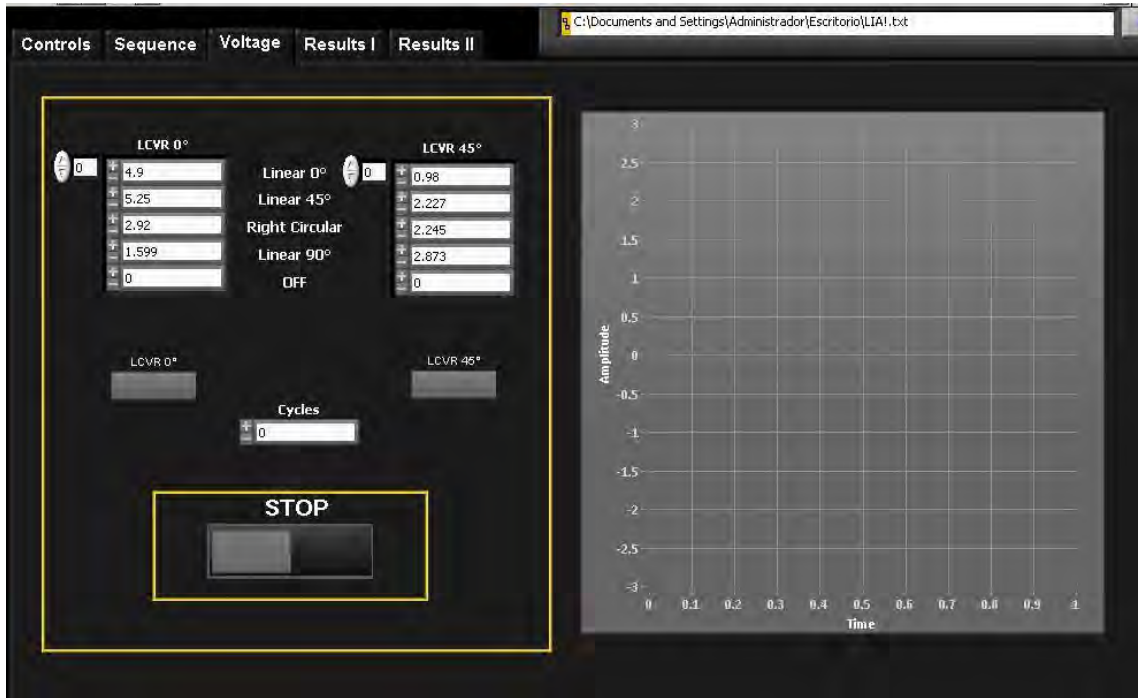
Figure 3.20 – Implementation and control panel of the voltage sequence for the LCVRs
