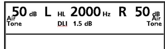
Picture 22 MA 52 display with DLI test
