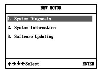
This menu is the main menu of this diagnostic scanner; all the diagnostic functions enter from this menu. Because of its importance, we will give a detailed description in the later section.
