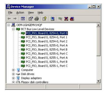
The specific low level devices found while installing PCI data acquisition cards is card specific. The table below shows what hardware will be detected for each type of PCI data acquisition card supported by the driver.
