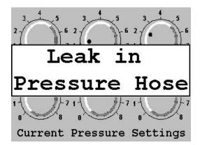
The resulting display is made possible assuming that screen 12 is triggered first, which will clear the display and add itself. Then screen 6 is triggered second. Since it is a cover screen, the fields from the first screen show through to the resulting display in any character positions not occupied by fields on the cover screen 6.
