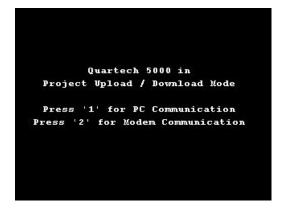
In the case of the 5000T, touching the screen anywhere while power is applied will bring the unit into its Project Upload/Download Mode. The following screen will appear:
