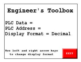
The Exit button is a screen trigger button assigned in Setup/OIT/General.
