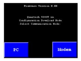
Select **PC** to download via a direct connect to the personal computer. Use **Modem** to download via a modem connection to the personal computer. Both require ScreenMaker software to be running on the personal computer.
