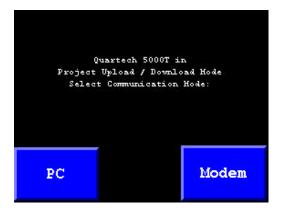
If an Upload or Download is desired for local connections press the 1 key for a 5000C unit or press **PC** for a 5000T and the unit will display the following:
