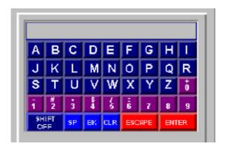
The Operator can either use the **ARROW** keys for navigational around the keypad, or the touchscreen. The **ESCAPE** and **ENTER** keys on the 5000C serve the same purpose as the escape and enter keys located on the pop-up keypad. The shift off key will act like a maintained selector, thus requiring a push-on push-off procedure.
