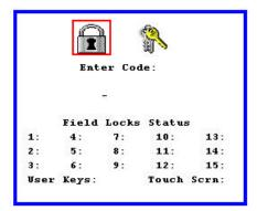
The operator can use the ARROW key to move the focus off of the Lock icon and onto the Unlock icon. At this time he/she can enter the four digit code to unlock/lock the specific field. The numbers listed below the Field Lock Status indicate what lock codes are enabled. In the example above, no field locks are enabled. An X would appear next to the number that had a lock enabled.
