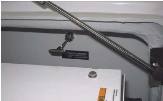
Lever pulled :Supply Diesel - Port tank
