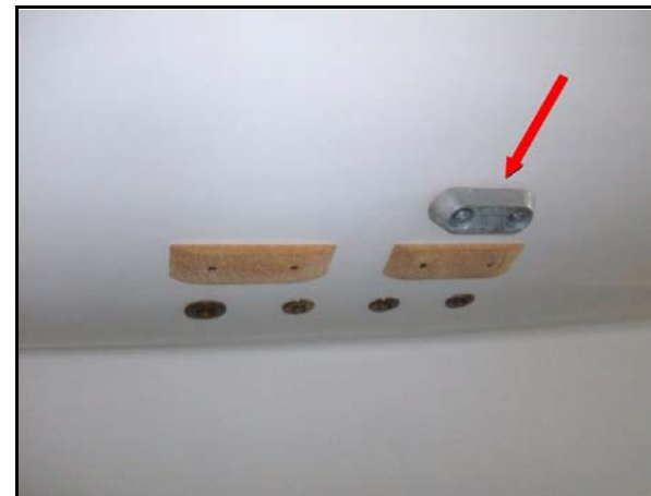
ANODE (On hull, under water line)
