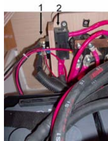
Lay out of: Port aft cabin 1. SHUNT - 100A 2. General fuse 12V - 100A
