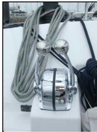
BILGE PUMP LEVER - ENGINE
