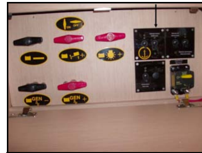
100A BREAKER (ELECTRIC WINCH DAVIT - OPTIONAL EQUIPMENT:)
