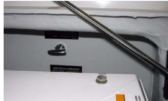
Lever pushed: Supply Diesel - Starboard tank
