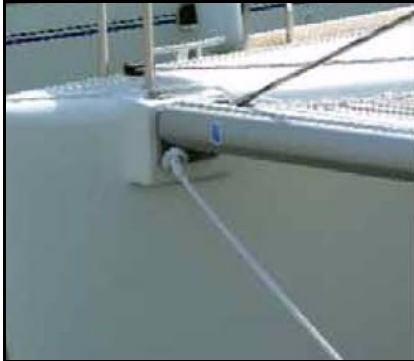
ATTACH THE BRIDLE TO THE FORWARD BEAM
