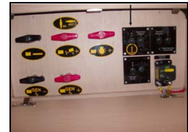
WINDLASS CIRCUIT BREAKER - 100A Port aft cabin
