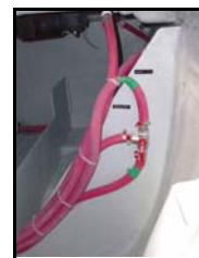
Selection valve - Fresh water / Sea water (Reference 2)
