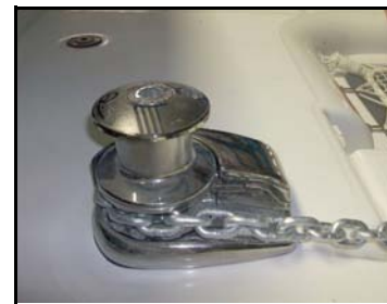
WINDLASS 12V 1000W Chain lifter 10mm diameter
