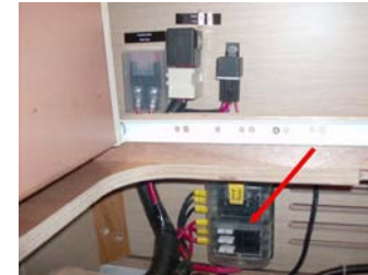
Lay out of: Port aft cabin (Under the bed) Pump - (25A) electric toilet
