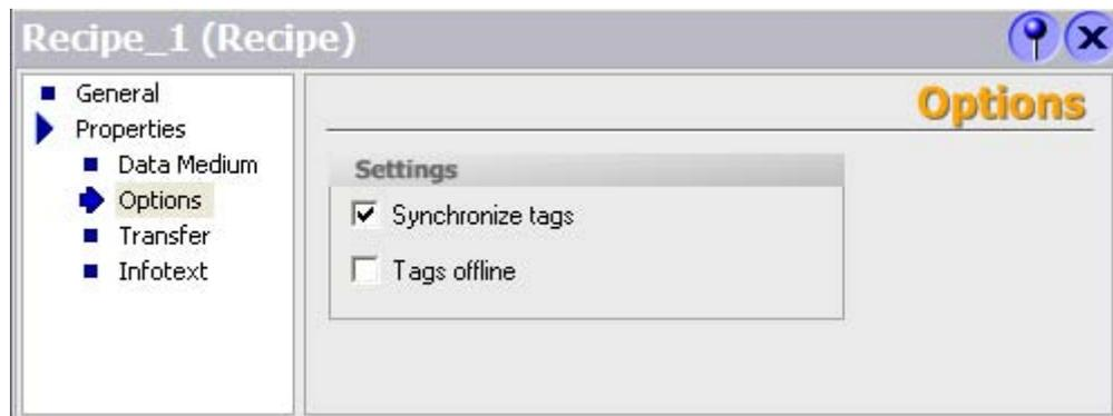
You must synchronize the tags in order to synchronize data between the tags of the recipe screen and the recipe data records displayed in the recipe view. Synchronization of tags is only possible in the enhanced recipe view.
