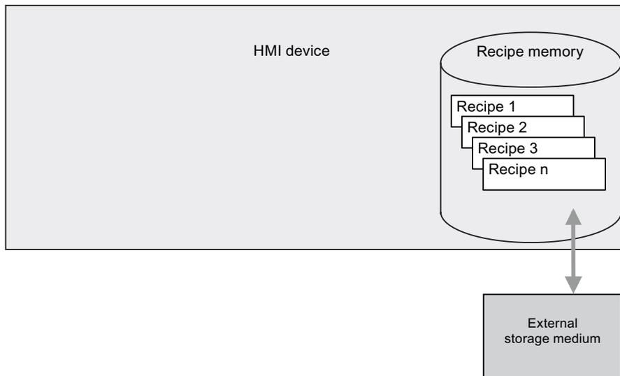
Recipe data records are exported from the HMI device recipe memory and are saved to a CSV file on the external storage medium. The records can be reimported from the storage medium to the recipe memory.
