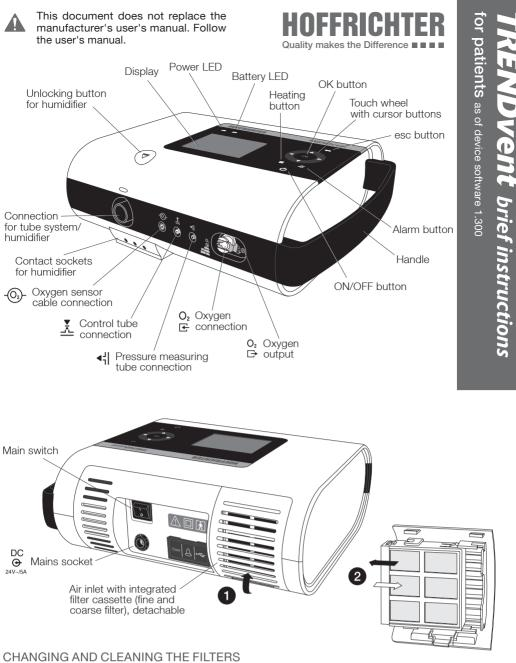
The coarse filter must be cleaned once a week. The white fine filter cannot be cleaned. It should be inspected visually weekly and replaced monthly or more frequently if heavily soiled.
