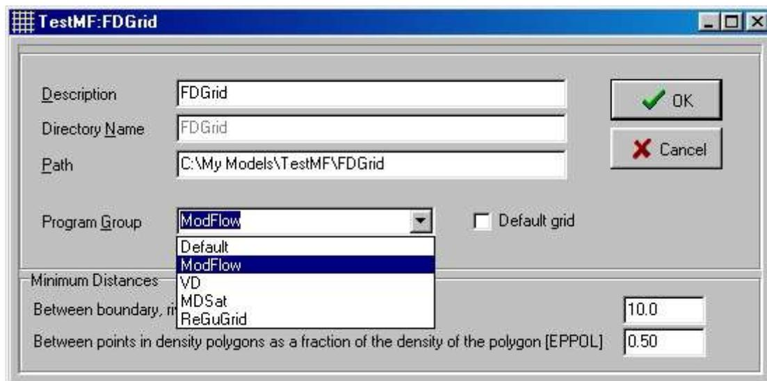
Monet is used as two-dimensional mesh generator for **Triwaco** when the simulation is carried out with ModFlow. Monet produces a [Tesnet compatible output](#) file with a number of additional sets that facilitate the generation of Modflow datafiles.
