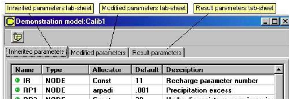
Double clicking on one of the parameters starts the graphical editor [DigEdit](#). For each of the parameters the user can create a new **map** and **par file** or modify the existing **map** and **par file**. These changes take place in the directory of the Initial data set the Calibration set is based on!
