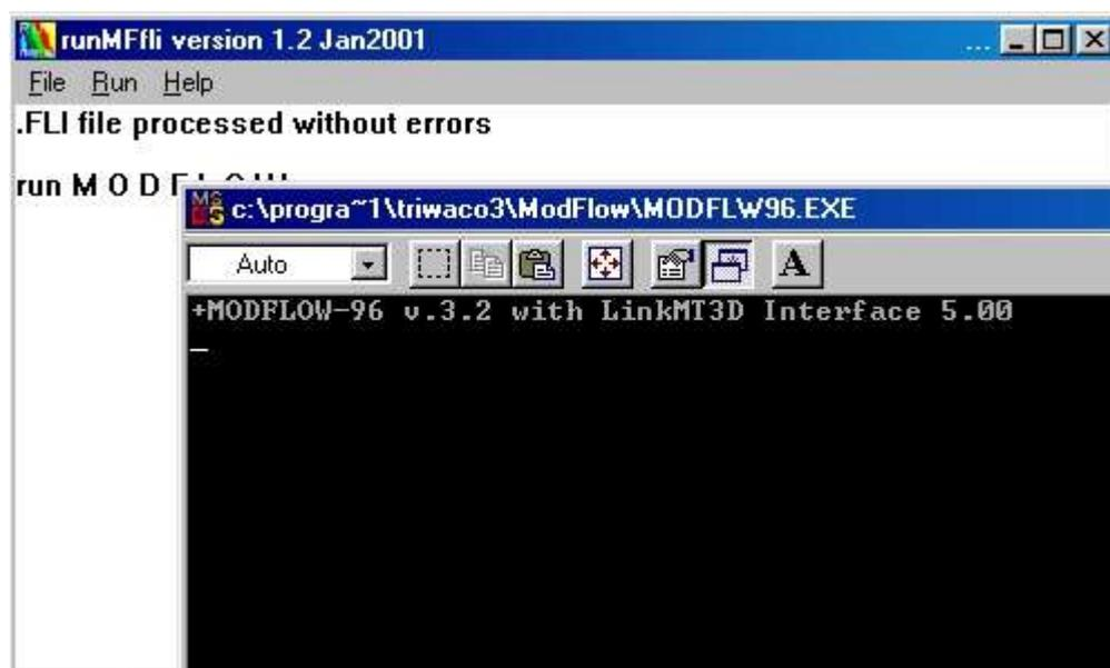
The simulation program produces different types of output files. **RunMFli** writes and converts the standard ModFlow output back into standard **Triwaco** output format (default file name **flairs flo**). All ModFlow files remain present. Some of these files contain information on the calculation process, errors encountered, (**flairs.flg**) others contain the calculation results using various formats (**flairs.flp**, **flairs.flo**).
