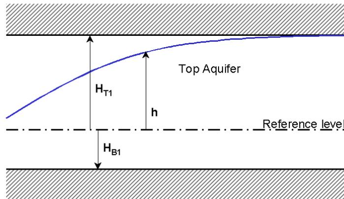
The aquifer's transmissivity is computed with the following assumptions:
