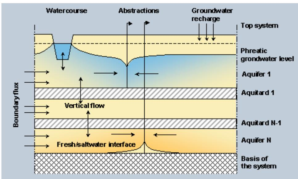
The recharge term ' $q$ ' comprises a number of different effects. In the program **Flairs**, ' $q$ ' is divided into four distinctive components, depending on the origin of the water:
