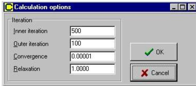
During calculations **Flairs** will pause and display a warning if the maximum number of linear or **inner iterations** is exceeded. If the user decides to continue calculations **Flairs** automatically doubles the number of inner iterations. For each **outer iteration**, the number of inner iterations will be checked.
