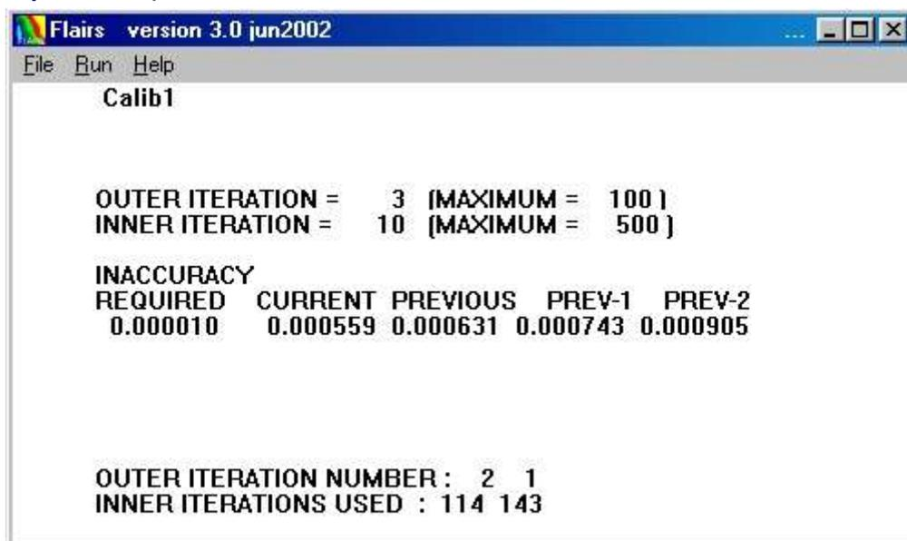
Triwaco computes groundwater heads/flow by iteration, starting from groundwater heads equal to 0.0. A quicker calculation process may be obtained if initial head values are used which are closer to the heads to be calculated. The initial head is often defined by the output of the former simulation result. Definition of the initial head is described in [par. 5.1.5](#).
