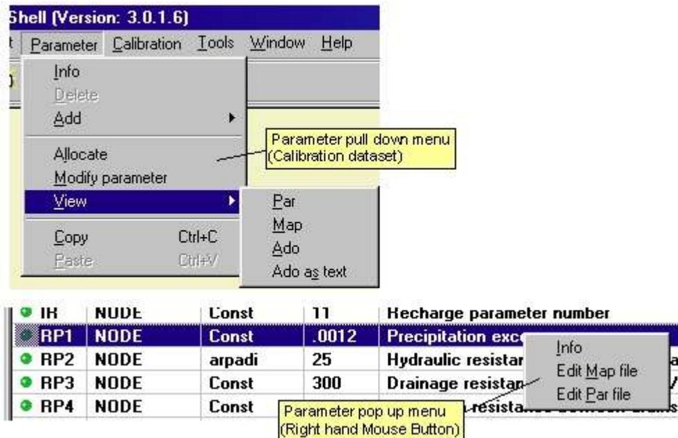
Selecting 'Modify parameter' moves the selected parameters from the 'Inherited parameters' Tab-sheet to the 'Modified parameters' Tab-sheet. The parameter's original par and map files (in the Initial data set's directory) remain unaffected and a new set of par and map files may be created. These files will be located in the Calibration data set's directory.
