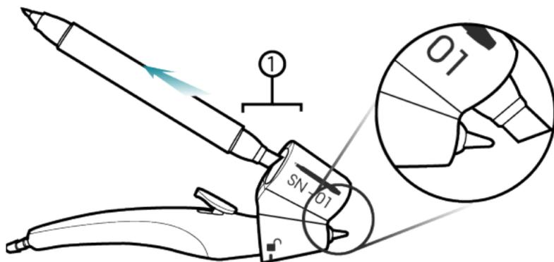
To remove the marker from the adaptor, (1) pull the marker straight out from the adaptor.
