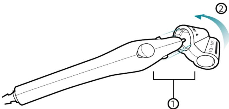
With the marker adaptor showing the “Arrow” icon (▲), (1) insert the marker adaptor onto the eBrush. Once in place, (2) twist the marker adaptor counterclockwise to lock the marker adaptor in place.
