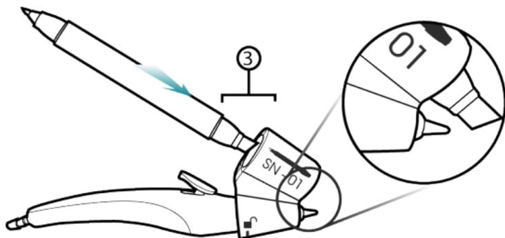
(3) Insert the desired marker into the adaptor. Some adjustment may be required to align the chisel point of the marker parallel to the eBrush nozzle.
