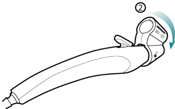
To change the marker adaptor, (2) twist the marker adaptor clockwise and remove while holding onto the eBrush.
