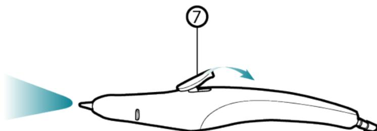
Pull back on (7) the eBrush trigger and hold to allow air flow.
