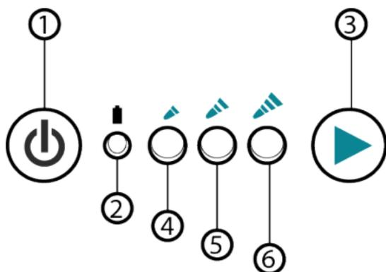
(1) Power Button to turn on or off the air compressor.
