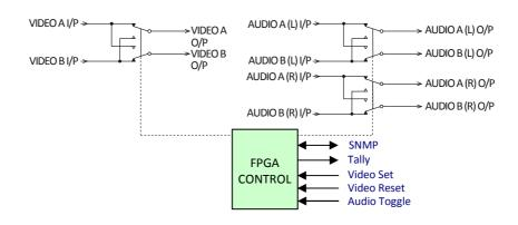
The AMS-4172 consists of one "video" and two "balanced audio" switches arranged as a changeover set with two inputs and two outputs. No terminations are provided on the board allowing the switcher to be used in a wide variety of applications and with signals of various types and impedances.
