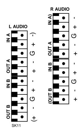
When wiring, be sure to keep phase of audio cables the same. The above connector will take either a balanced input, balanced output audio (or data (RS-232, RS-422, etc.)) signal, or two unbalanced audio signals, where the ground connectors are commoned together and the two unbalanced audio signals connected to each of the +/- phase connections.
