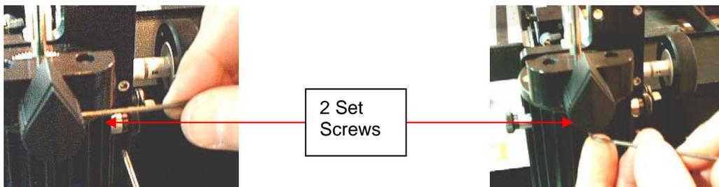
8. Carefully install the Pick Shroud onto the Reflow Head Assembly. Make sure that the Vacuum Pick moves freely when turning the Vacuum Pick Control Knob.
