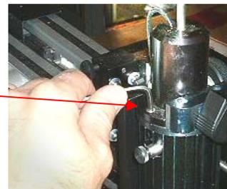
4. Carefully lift the Pick Shroud from the Reflow Head Assembly.
