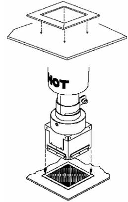
12. Using the Vacuum Pick Adjustment Control Knob, adjust the vacuum cup to a point where the bottom of the cup is flush with the bottom edge of the nozzle.
