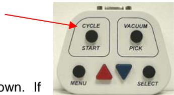
15. The LCD will display the remaining cycle (“Reflow”) time counting down. If the Auto Vac is selected in the Setup Mode, the vacuum will automatically activate 5 seconds before the end of cycle.
