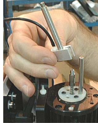
6. Before installing the Theta Knob Assembly, be sure to properly line up the Vacuum Pick Control Knobs.
