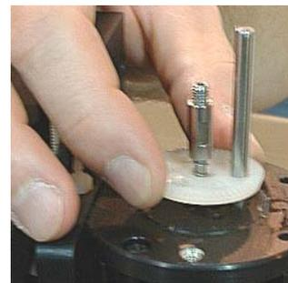
5. Insert the Manifold Vacuum Assembly and tighten the vacuum pick with a  $7/32$ " open-end wrench. Must be snug but do not over tighten!
