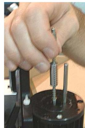
12. Remove the E-Clip and slide the Springs and Gear Rack from the Vacuum Tube. With the exception of the Vacuum Tube, these parts will be reused on the new Vacuum Tube.
