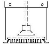
**CAUTION:** Be sure to keep the distance between the vacuum cup and the component at a minimum. Only a slight gap is required for the component to be raised from the PCB.
