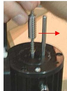
3. Use the Vacuum Pick Control Knob to verify engagement of the Vacuum Tube Assembly.
