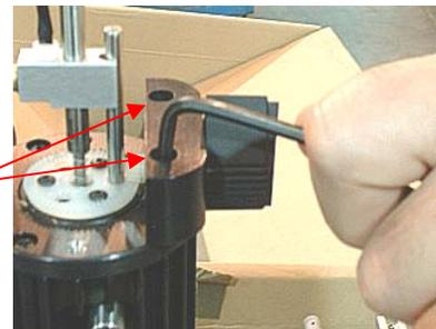
7. Loosen the vacuum pick with a 7/32" open-end wrench.
