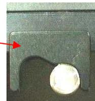
**NOTE:** The tension slide is used to apply a small amount of tension on the PCB assembly once the Board Holder Rails are secured in place. This additional tension will help further retain the PCB in the fixture.
