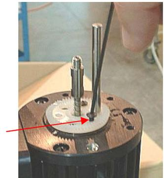
10. Gently lift the Beveled Gear from the Reflow Head.
