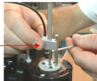
8. Carefully lift the assembly from the vacuum tube.
