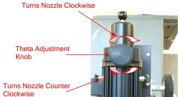
Theta Adjustment - Moves the Reflow Head up to 10° in either direction.
