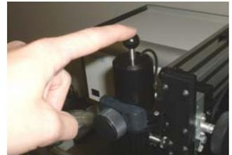
16. Using the Vacuum Pick Height Adjustment Control Knob, adjust the vacuum cup to a point where the bottom of the vacuum cup is flush with the bottom edge of the nozzle.
