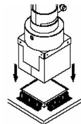
c) Contacting the BGA component when using a V-A-N nozzle.
