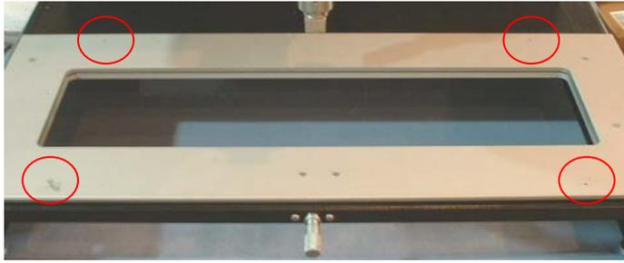
2. Install the rail assembly using the four flat head screws and the 5/64" hex key.
