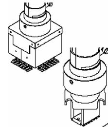
17. Ensure that the Nozzle is square to the PCB. (See the section on Reflow Head Positioning on page 20 if an adjustment is needed)
