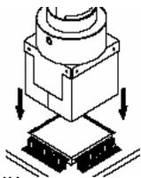
14. Press and release the Cycle Switch to activate heat cycle.
