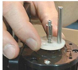
11. Carefully remove the vacuum tube assembly from the Reflow Head.
