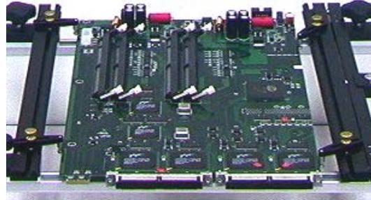
1. Loosen the Rail Adjustment Knobs.
