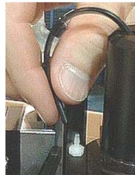
10. Turn the knob clockwise to install it on the shaft. Hold the shaft when tightening in order to keep the shaft from rotating.
