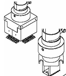
13. Ensure that the Nozzle is square to the PCB. (See the section on Reflow Head Positioning on page 20 if an adjustment is needed)
