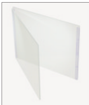
Fig 6. Pre-assembled hinged Gel Casting Cassette for 26 × 20 cm lab-cast gels. The differential plate heights ease IPG strip loading. The two glass plates are joined along the left edge by a silicone rubber hinge. Sticky vinyl spacers, 1.0- or 1.5-mm thick, are glued on each edge of the long plate. Close and open the cassette like a book.
