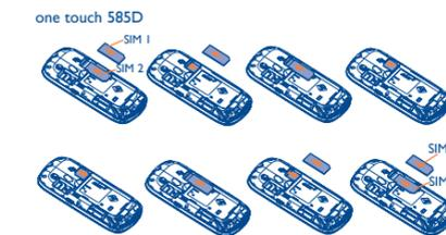
Place the SIM card with the chip facing downwards and slide it into its housing. Make sure that it is correctly inserted. To remove the card, press it and slide it out.
