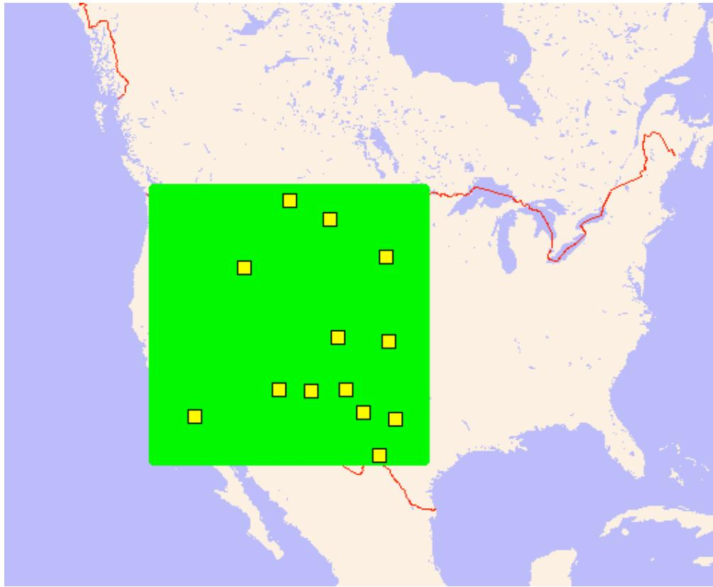
The green circles represent the locations of the travel-time grid nodes. The yellow squares represent the station locations. The grid should cover the entire region where earthquakes are likely to occur. However, there is a tradeoff. If the grid is coarse, dbgrassoc will run fast, but the preliminary eq locations will be less accurate. If the grid is fine, dbgrassoc will run slower, but the initial earthquake positions will improve.
