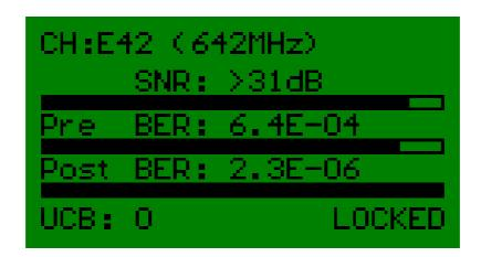
Hopefully, but not always, the digital readout; BER (bit error rate) and SNR (signal noise ratio) will correspond well with the analog setting of the antenna.
