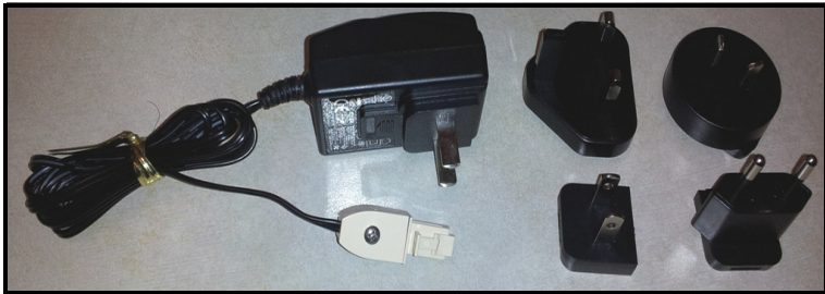
Figure 4: M2831 AC adapter and M2835 plug set
