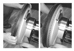
Place the dust skirt in the intended notch on the rubber strip.
