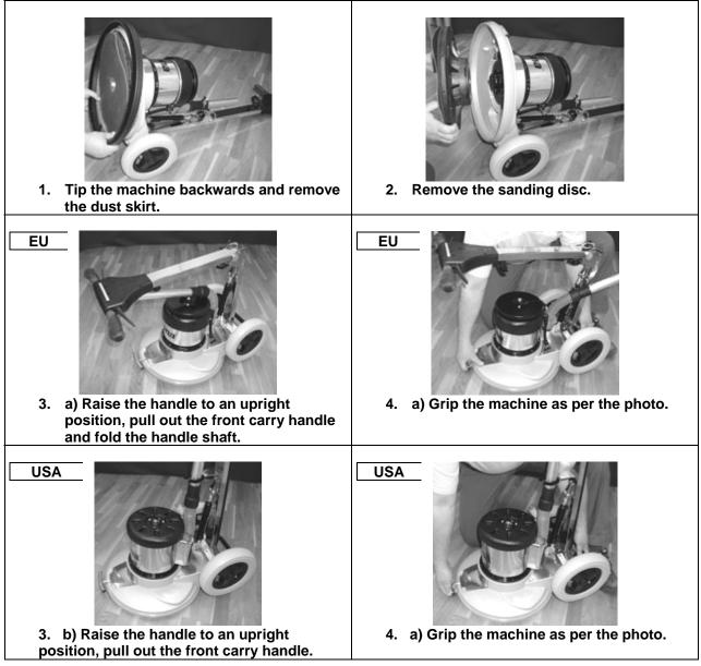
NOTE! Always remove the dust skirt and the sanding disc before transportation!
