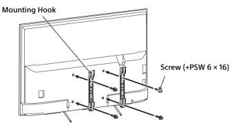
**3** Make sure that the wall has enough space for the TV and is capable of supporting a weight of at least four times that of the TV. Refer to the following table on installing the TV to the wall. See page 20-22 (Specifications) for the TV's weight.
