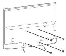
2 Attach the Mounting Hook using the four screws supplied with the Wall-Mount Bracket.
