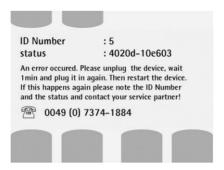
This error message appears as soon as the SpasmControl is activated 25 times at short intervals or if the motor was locked for a period of 3 minutes. Please pull the mains plug out of the plug socket and put it in again. Then please check if the motor power is adjusted too low or if the pedal radius is adjusted too high in relation to the patient's condition.
