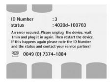
This error message appears if the pedals are moved before the MOTOmed letto2 is ready for starting up (the green small lamp at the operating panel must burn permanently). Please pull the mains plug out of the plug socket, put it in again and wait until the green light at the operating panel is burning permanently.
