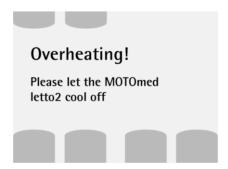
The MOTOmed letto2 overload detection is responding. Please wait several minutes until the motor has cooled down and the buttons of the operating panel react again. If overheating occurs twice, please interrupt the training for approx. two hours in order to let the motor cool down completely.
