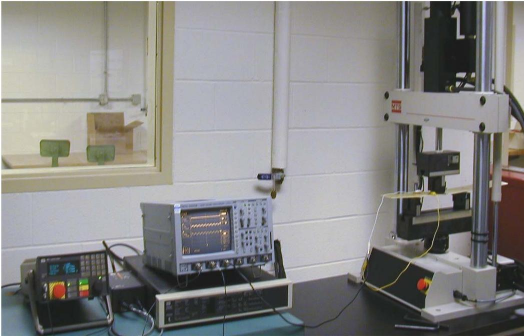
Figure 6.19 Experimental setup for power harvesting of sensors bonded on the beam
