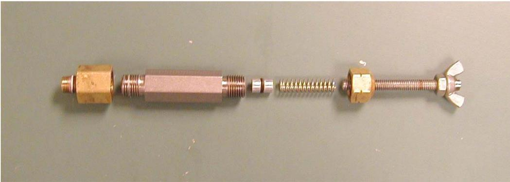
Figure 3.3 Injector Assembly
