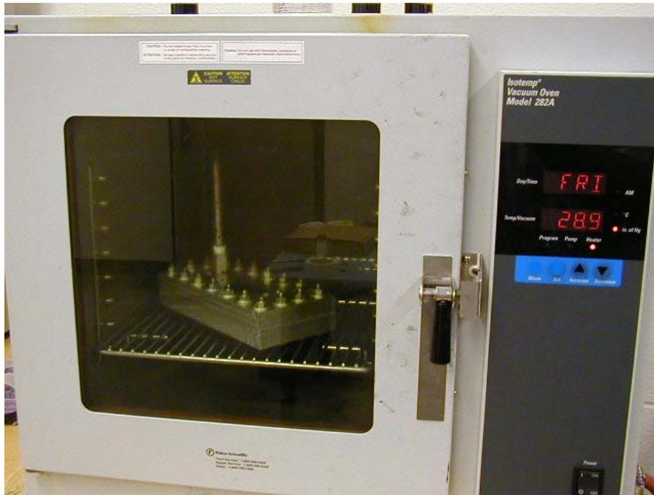
Figure 3.5 Curing for the AFC Sensor
