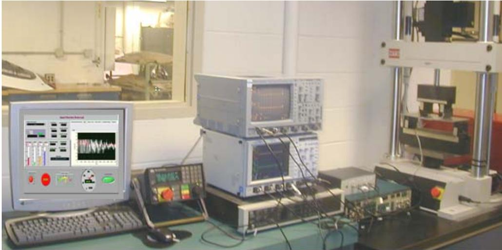
Figure 5.7 Setup of MTS machine and LabVIEW data acquisition system to test the riveted aluminum plate
