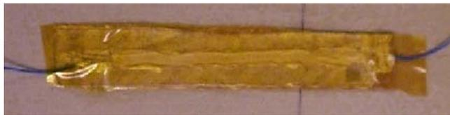
Figure 3.12 Manufactured Active Fiber Composite Sensor
