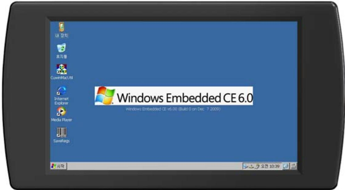
The CUWIN's front panel features an 800x480 color touch screen capable of receiving input from a human user, by touching the screen, and displaying colorful information.
