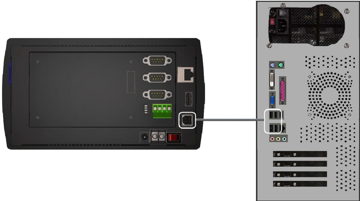
2. Using a USB cable, connect the CUWIN to the PC.
