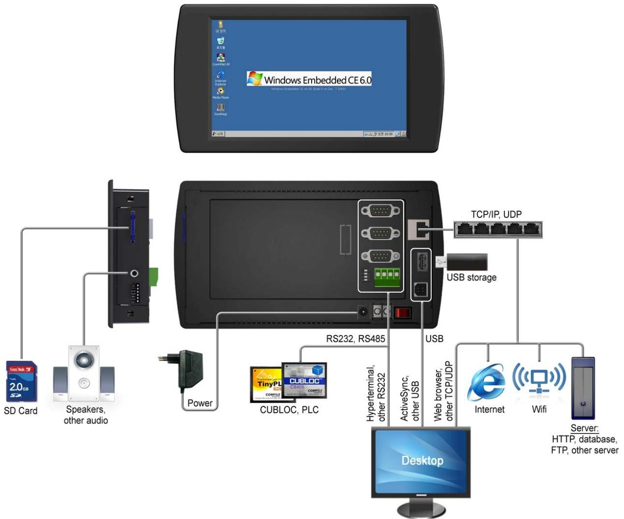
The CUWIN translates input from a human user to signals that electronic devices can understand, and receives signals from those electronic devices, translating them to colorful output that the user can understand. Thus, the CUWIN serves as a Human Machine Interface(HMI).
