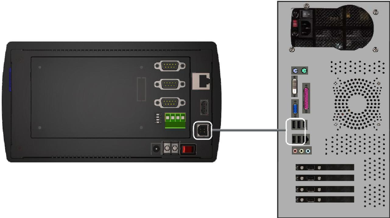
9. Using a USB cable, connect the CUWIN to the PC.
