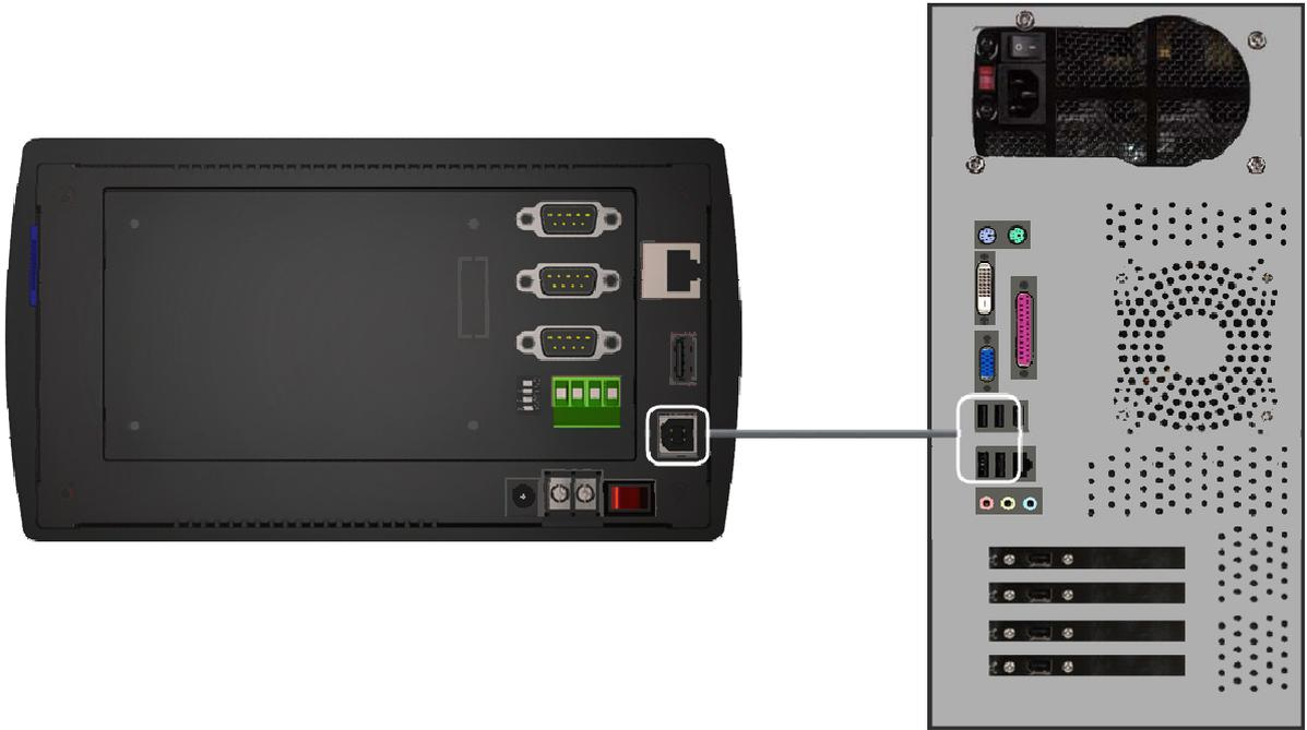
12. Using a USB cable, connect the CUWIN to the PC.
