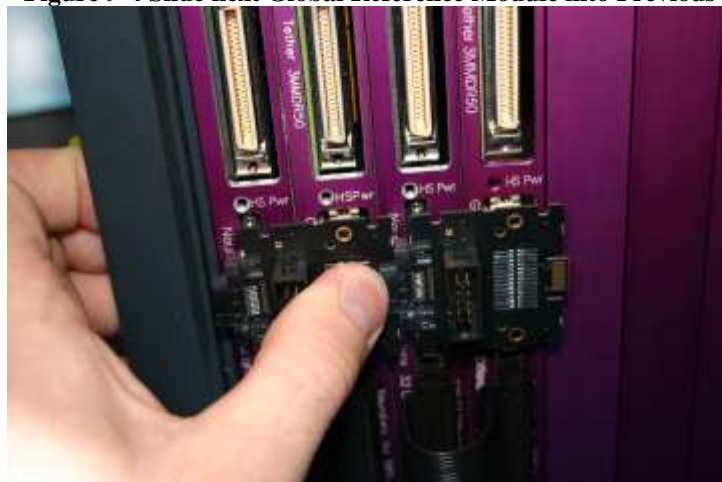
Figure 9-5 Connect Global Reference Module to DRS Board
