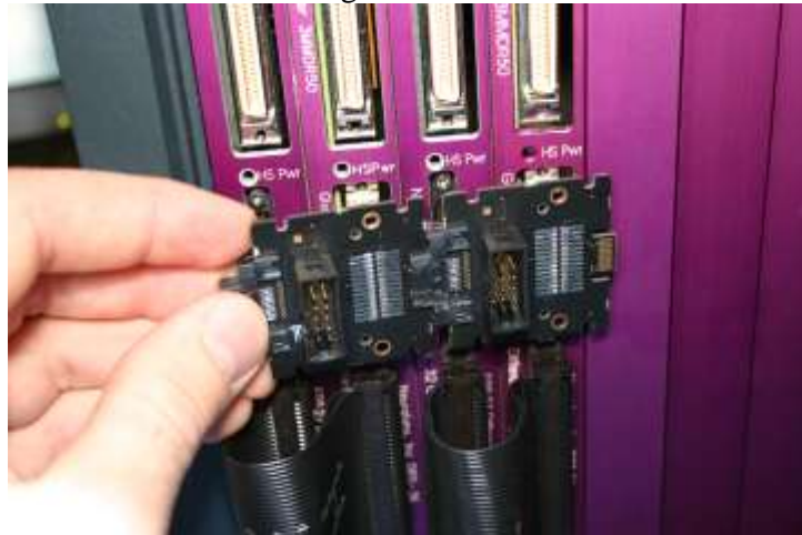
Figure 9-4 Slide next Global Reference Module into Previous
