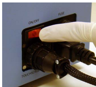
Fig. IV-F-3. Turn on main power.
