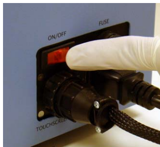
Fig. III-C-3. Turn on main power.
