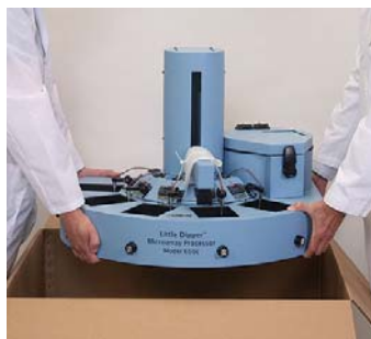
Fig. III-A-1. Lift by the base.
