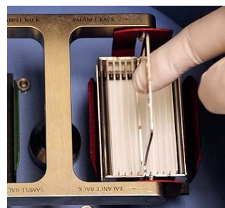
Fig. IV-A-8. Load balance rack.
