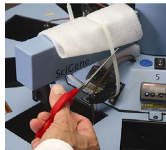
Fig. III-A-2. Cut tie wrap.
