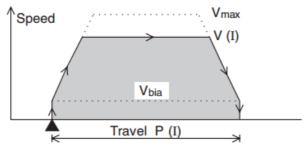
When the start command is given, the motor accelerates up to the operating speed V(I) (BFMs #20 and #19), then decelerates and stops in the set position P(I) (BFMs #18 and #17).
