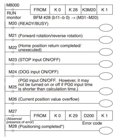
\* When a drive amplifier for a stepper motor without the positioning completed output is used, this signal can be used for recognition of positioning completed and the next operation can be started.
