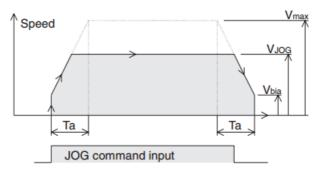
Any value between the bias speed  $V_{bia}(BFM~\#6)$  and the maximum speed  $V_{max}(BFMs~\#5)$  and #4) is valid as the command speed  $V_{JOG}$  (BFMs #8 and #7). The acceleration/deceleration time Ta(BFM #15) is the time between  $V_{bia}$  and  $V_{max}$ .  $V_{max}$ ,  $V_{bia}$  and Ta are equivalent in the operation modes described later.
