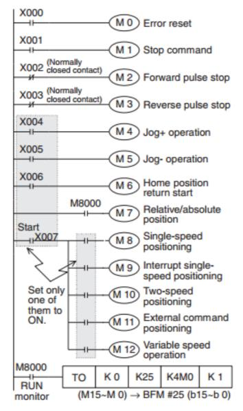
• Error can be reset by forcedly turning on/off the peripheral unit. The input X000 does not have to be used.
