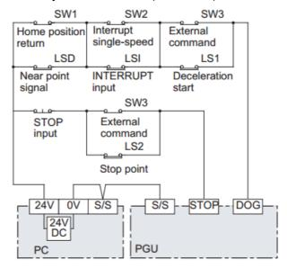
Input switches SW1 to SW3 are selected in accordance with the type of operation.
