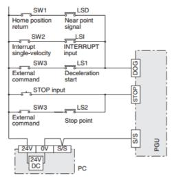
Input switches SW1 to SW3 are selected in accordance with the type of operation.
