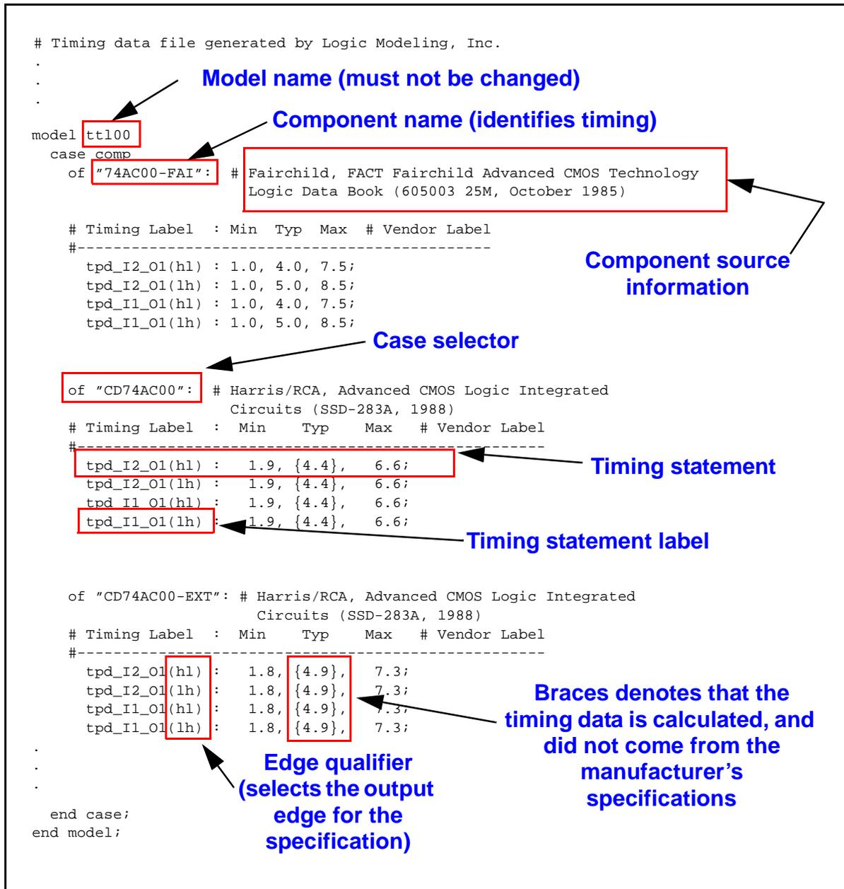
Figure 21: Annotated Timing Data File Model Block
