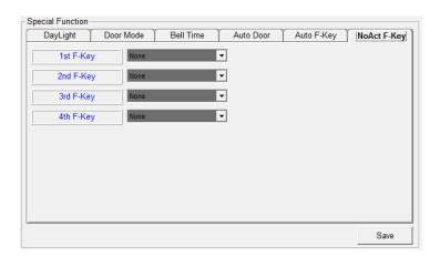
No Act F-Key: for not activating the door operation relay if entrance authentication occurs using the function key set at the relevant window. This can be mainly used if door should not be opened while checking attendance.
