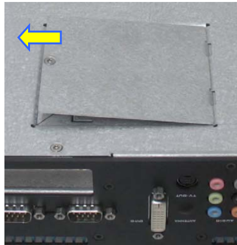
Fig. 23: Detail - lifting up the CF slot access cover
