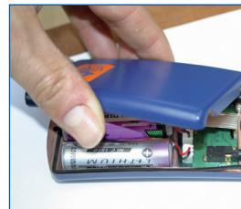
VI. Close Main Box and lock it by the 2 fixing screws.
