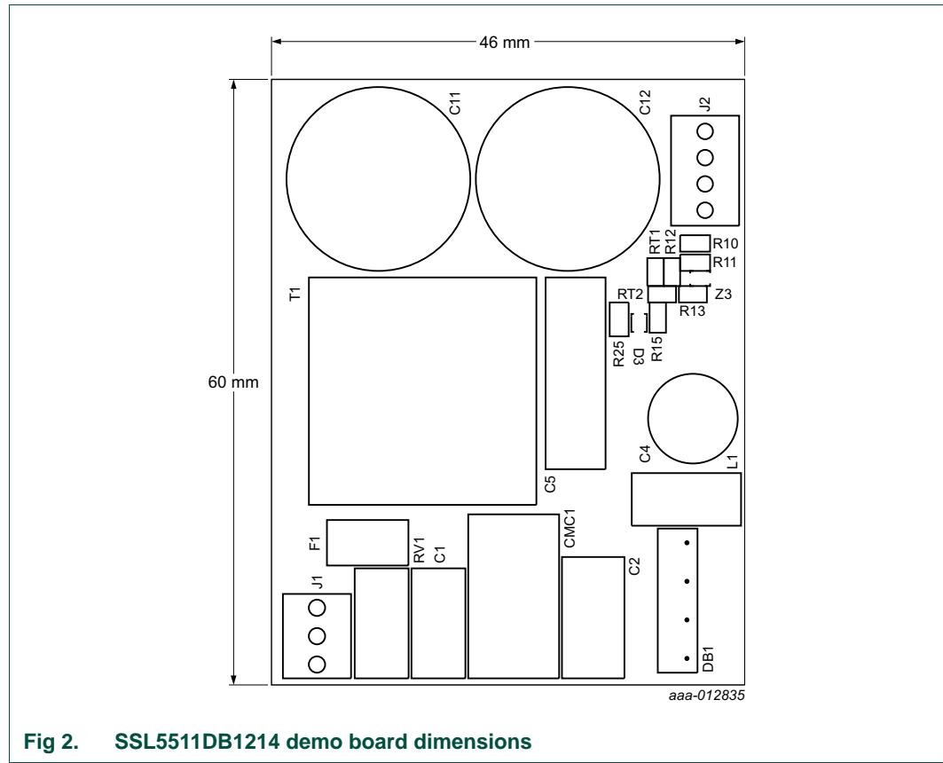
**Fig 2. SSL5511DB1214 demo board dimensions**
