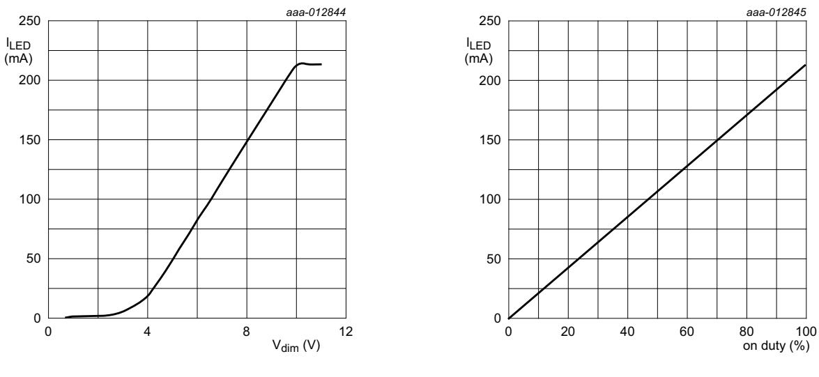
Fig 9. Output current as a function of dimming signal
