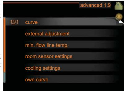
different outdoor temperatures here. If there is access to cooling the same settings can be made for the cooling curve.
