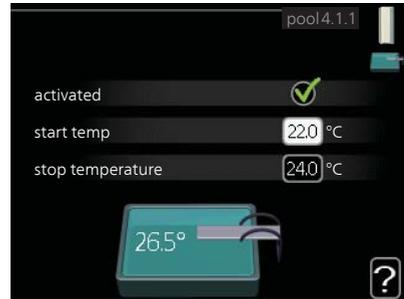
Select whether the pool control is to be activated, within what temperatures (start and stop temperature) pool heating must occur and how many compressors may work against the pool at the same time.
