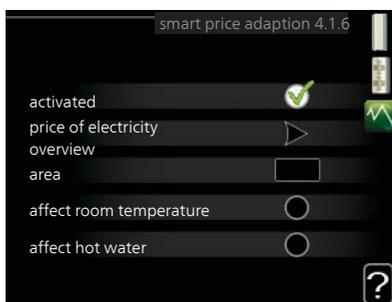
Activate smart price adaption by highlighting the function and pressing the OK button. When smart price adaption has been activated, the settings that can be made are displayed. To select which selectable functions are to be permitted or not you highlight the function using the control knob and press the OK button.
