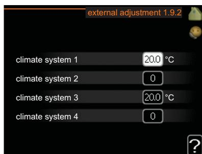
Connecting an external contact, for example, a room thermostat or a timer allows you to temporarily or periodically raise or lower the room temperature while heating. When the contact is on, the heat curve offset is changed by the number of steps selected in the menu. If a room sensor is installed and activated the desired room temperature (°C) is set.
