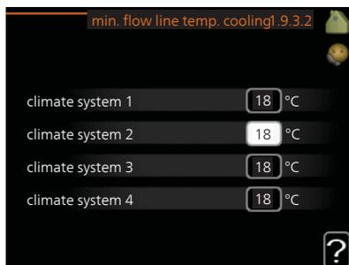
In menu 1.9.3 you select heating or cooling, in the next menu (min. supply temp.heating/cooling) set the minimum temperature on the supply temperature to the climate system. This means that SMO 40 never calculates a temperature lower than that set here.
