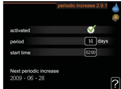
To prevent bacterial growth in the water heater, the heat pump and any additional heater can increase the hot water temperature for a short time at regular intervals.
