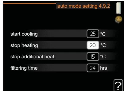
When the operating mode is set to "auto", the control module selects when start and stop of additional heat and heat production is permitted, dependent on the average outdoor temperature.
