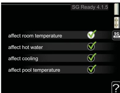
With low price mode on "SG Ready" the stop temperature of the hot water is set as high as possible at only compressor operation (immersion heater not permitted).
