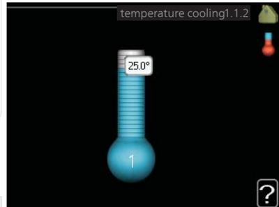
The number of steps the value has to be changed to achieve a degree change of the indoor temperature depends on the heating installation. One step is usually enough but in some cases several steps may be required.
