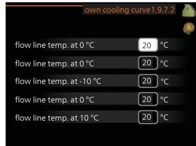
Create your own heating or cooling curve here, by setting the desired supply temperatures for different outdoor temperatures.
