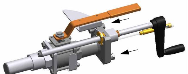
⇒ **Secure the two security screws properly**
