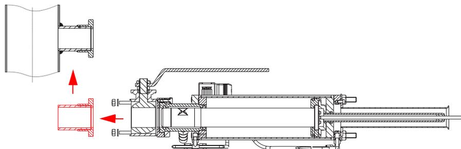
8. Remove the flanged weld-in stud from the cleaning device and weld the flanged weld-in stud to the pipe, according to section 3.2.4.
