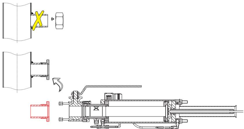
26. If the existing TCT-2301 is mounted with a flanged weld-in stud, remove the delivered weld-in stud from the cleaning device and mount the PCD-1000 to the existing flanged weld-in stud.
