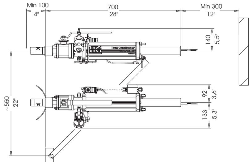
The installed device is approx. 700 mm (28 in) long. You will need at least 300 mm (12 in) to remove the device from the valve arrangement. The cleaning device weighs approx. 9.5 kg (21 lbs) including the TCT-2301 probe.
