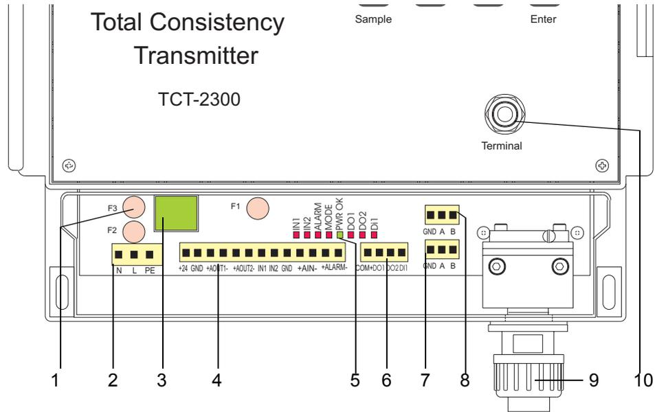
7. Switch on the main power on the electronics card. The power LED should now light up. See fig 25. If not, check first the connections and then the 2 AT fuse for the power supply located inside the electronics box.
