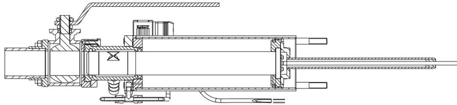
14. Push the probe and piston into the cylinder. Make sure the guide ring (10) is in position.
