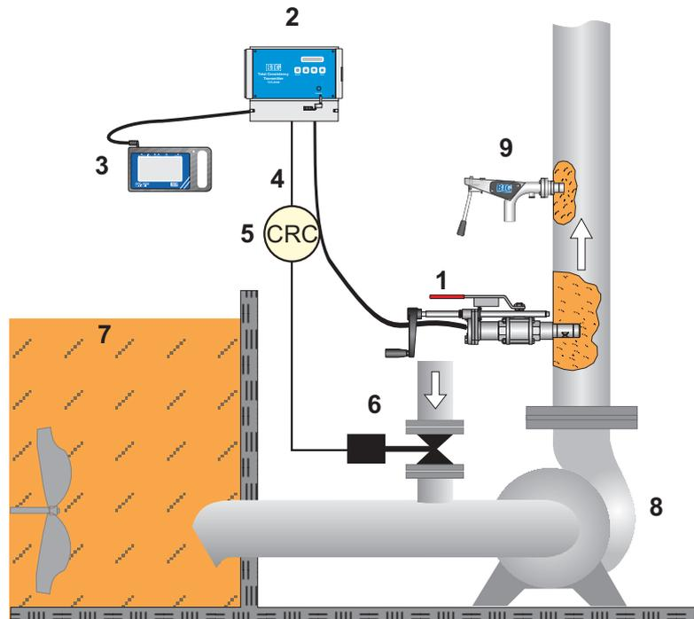
The system consists of a probe (1) connected by an optical fiber to an electronics box (2). The probe contains only optical fibers. A ball valve arrangement that is welded to the pipe system makes it possible to remove the probe without interrupting the process.
