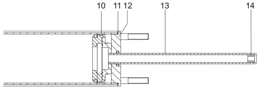
8. Remove cylinder flanged end (12) and pull out piston with guiding rod (13). Keep track of O-ring (11) and guide ring (10).
