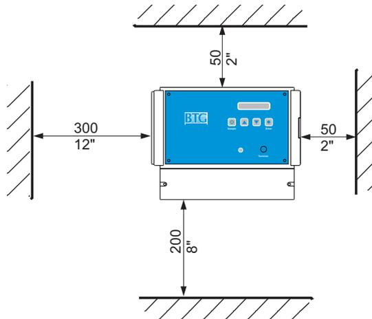
Install the box in a position where it will be protected from mechanical damage.
