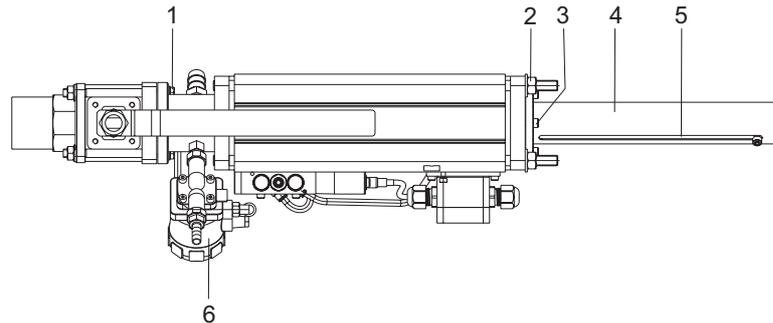
1. Loosen the screws (3) that holds the protective sleeve (4) fixed.
