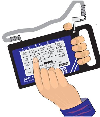
When the terminal is not in the wall terminal holder, place it on your left forearm (for right-handed users) and hold it securely using the hole in the handle. This is the most practical and safest way of using it, you can work properly without damaging the terminal.
