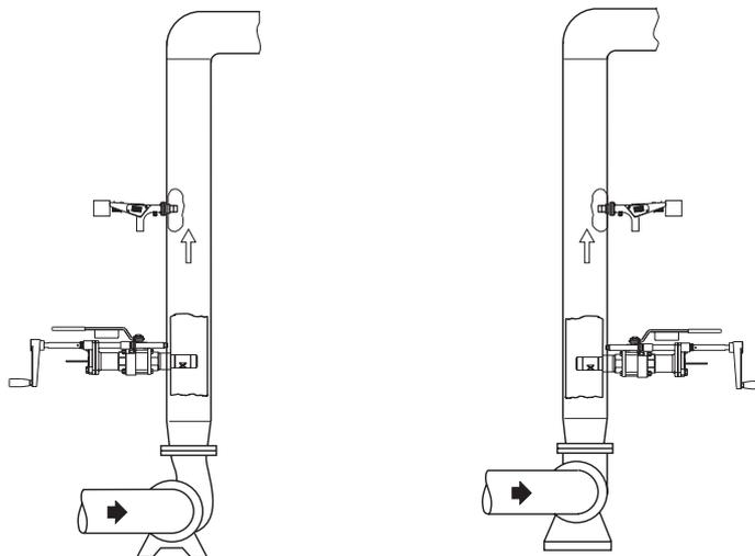
**Fig 9** Installation of the probe near a pipe elbow
