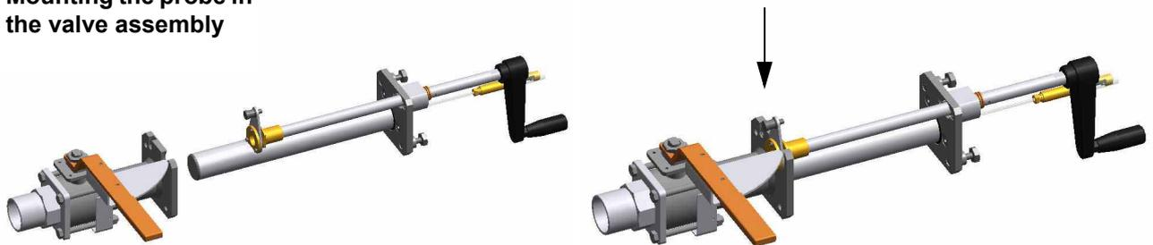
5. Open the ball valve and insert the probe by cranking the handle.
