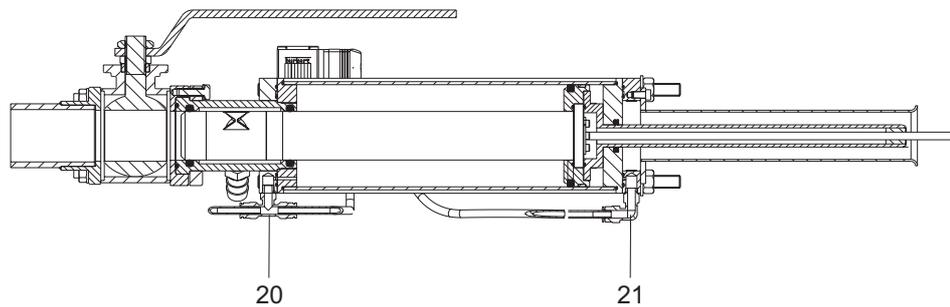
15. Mount the cylinder flanged end (12), the rear cylinder flanged end (6), and the protective sleeve (3), to the cylinder. Make sure that the O-rings (7, 8, and 11) are in their proper positions, and that the nipple (21) on the rear cylinder flanged end are positioned on the same side of the cylinder as the nipple (20) on the front cylinder flanged end. The parts must be pulled over the optic cable.
