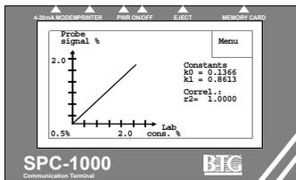
The probe signal is displayed as a function of the set measuring span xx - xx%. Probe signal points within the predetermined measuring span are displayed. Note that activated calibration points outside the measuring span affect the correlation.
