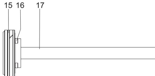
10. Loosen the screws (16) and separate the piston (15) and guiding rod (17) from each other.
