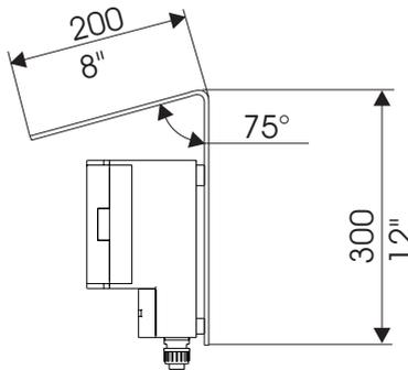
The electronics box is equipped with three attachment lugs and should be bolted to a wall.
