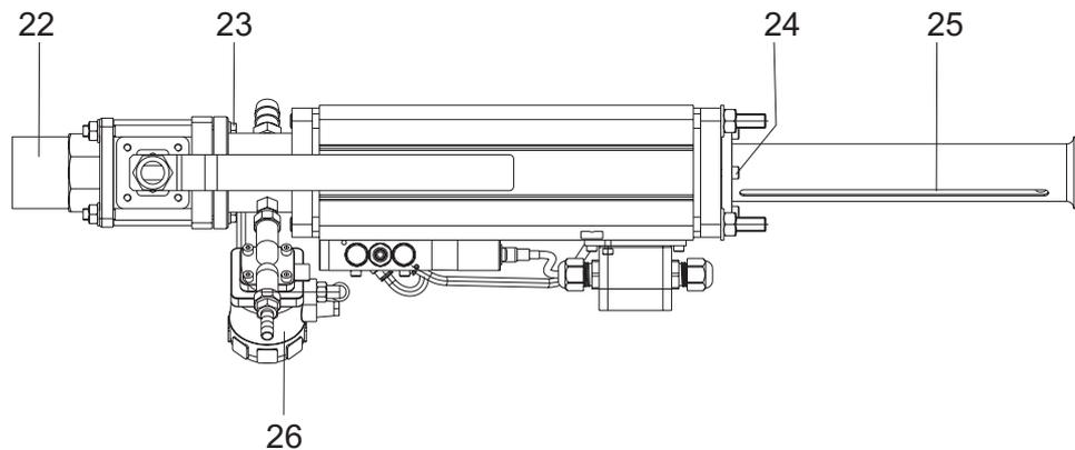
18. Loosen the screws (24) and turn the protective sleeve until the screw hole on the guiding rod is visible through the slot (25).
