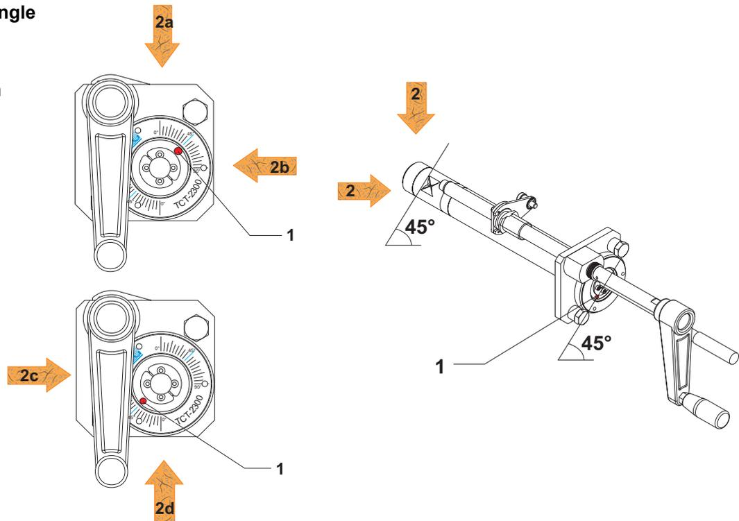
If the angle is not correct, loosen the three screws that hold the probe flange and adjust the probe so that the punch mark on the probe is at the 45° line on the scale. Tighten the three screws properly. A suitable allen key is included in the delivery.
