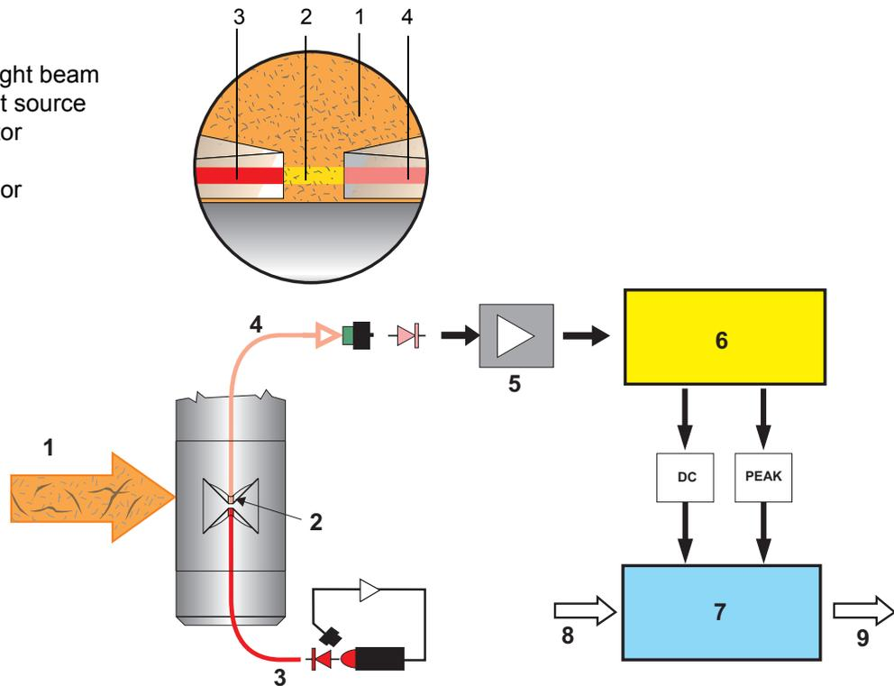
The TCT-2301 employs the patented peak method for measuring total consistency of pulp suspensions. This technology is based on the fact that suspensions contain both large and small particles. Large particles are typically fibers and small particles are fillers and fines.
