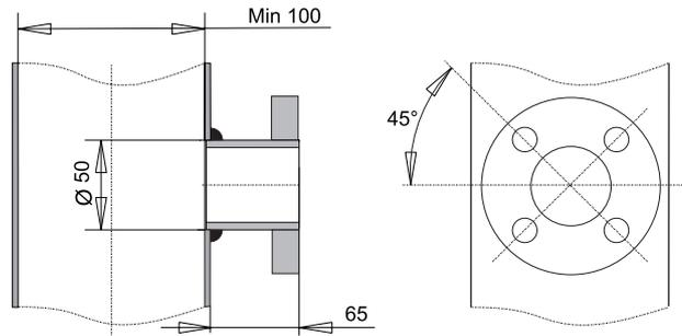
4. Make sure the weld-in stud is aligned to the pipe. See fig 12.
