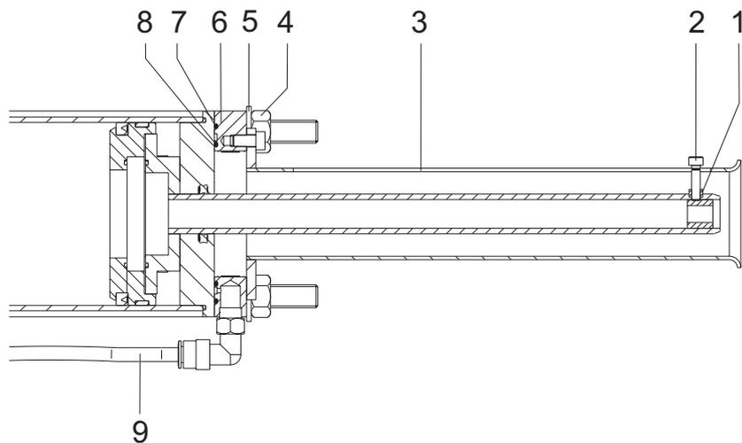
5. Unscrew and remove the screw (2) and the nut (1).
