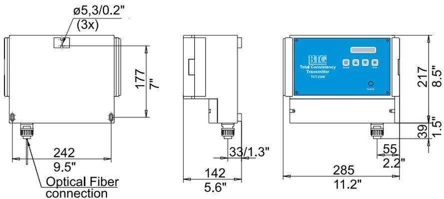
**Fig 18 Electronics box clearances**
