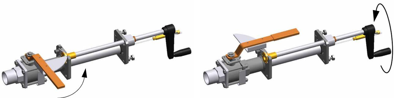
6. Secure the probe in inserted position with the two security screws
