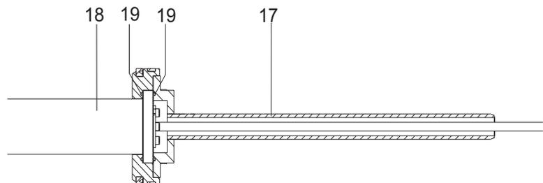
11. Insert the probe (18) in the piston (15) and the fiber cable in the guiding rod (17).
