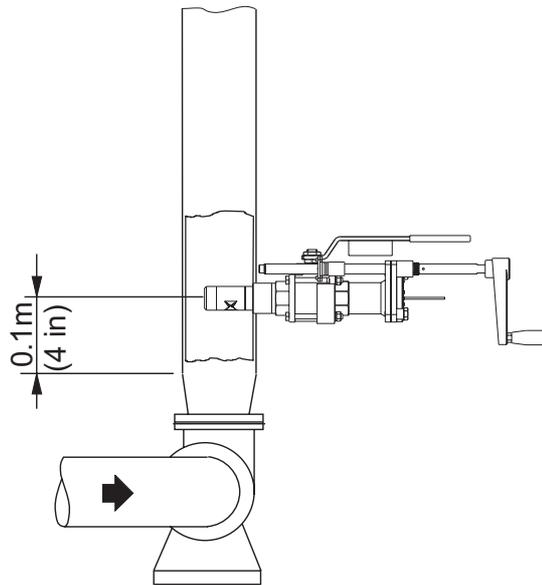
⇒ **Minimum recommended flow velocity: 1 m/s (3.3 ft/s).**
