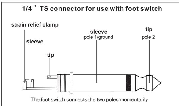
Fig. 4.1: 1/4" TS connector for foot switch
