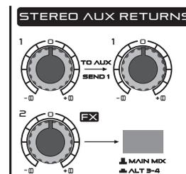
Fig. 2.9: Stereo aux return controls
