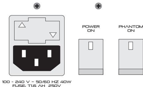
Fig. 2.15: Voltage supply and fuse
