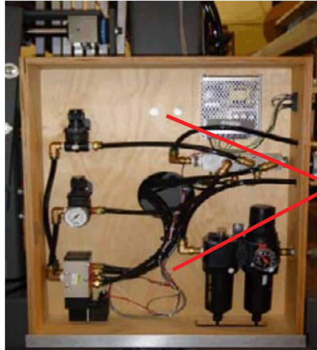
three mounting bolts for the Air Shuttle Control Box
