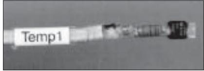
**Figure B-6: Temperature plus Humidity Sensors.**
