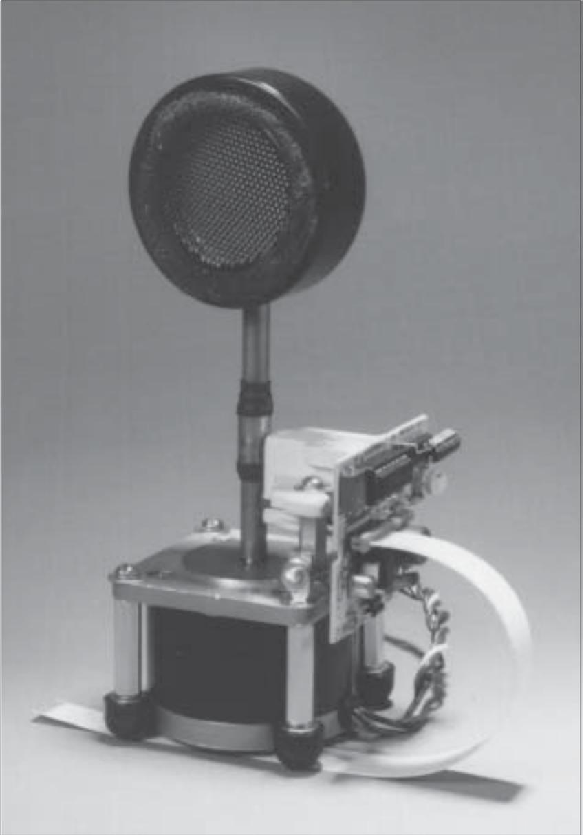
**Figure A-7: RADAR Mechanical Assembly**
