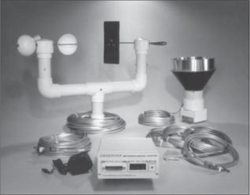
**Figure B-1: The Observer Meteorological Station.**
