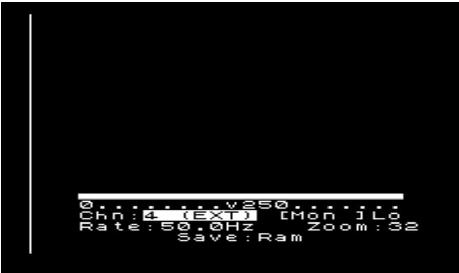
The screen is divided into a logging region and a control region. The bottom of the screen is the control region and occupies 160x128 pixels (in hi-res mode) or 50x32 pixels (in lo-res mode). At the bottom of the logging region is the sample scale and a 'v' or '^' symbol to let you know which region you're using.
