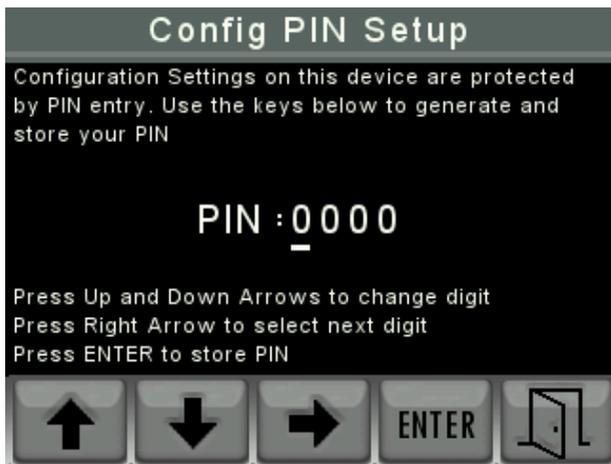
The user can use the “UP” and “DOWN” arrows to change the value of the underlined PIN number and then use the “RIGHT” arrow to choose the next number to change. When the desired PIN number has been chosen pressing the “ENTER” key will store it and then pressing the “EXIT” key will return to the settings menu.
