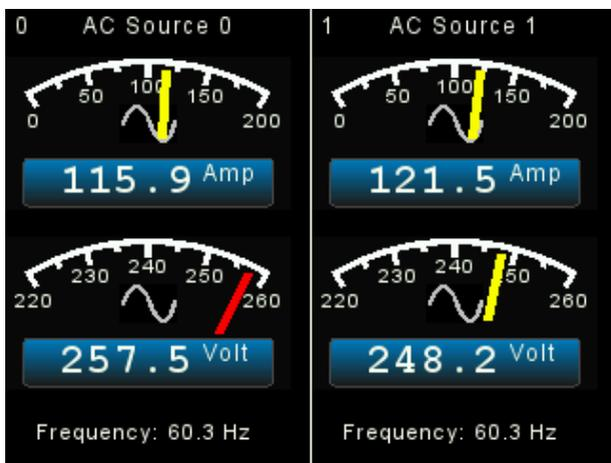
Repeated pressing of the “ACPWR” button will display the next two AC sources to a total of 16 sources.
