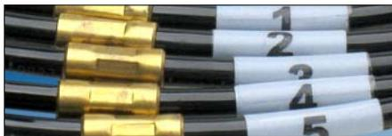
Metric cables have 0.5m graduations with numeric depth labels every meter. English cables have 2 foot graduations with depth labels every 4 feet. Graduations are measured from top wheels of probe. The four-conductor cable has a Kevlar strain member, and polyurethane jacket.
