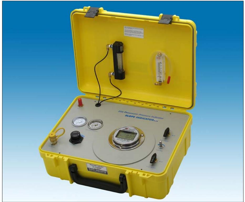
256 Pneumatic Pressure Indicator with Digital Gauge
