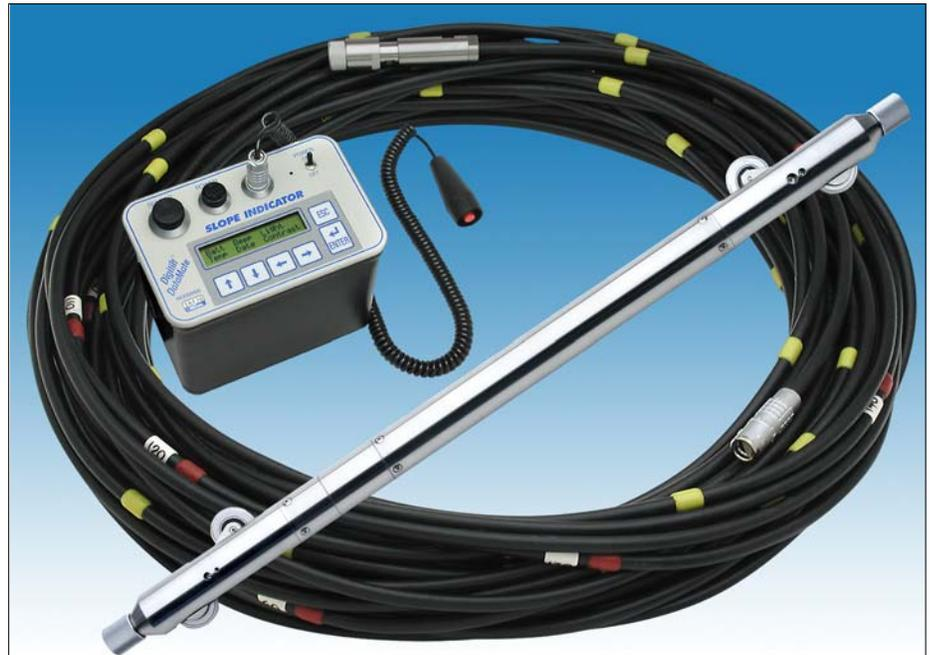
The probe is then reversed end-for-end and drawn through the casing a second time. Tilt measurements from the reversed probe are used to eliminate any error due to sensor bias and to generate checksums for validating the survey.
