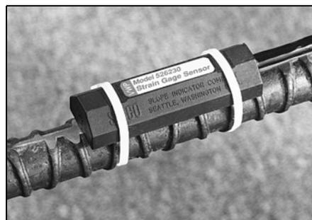
Spot-weldable strain gauge installed on reinforcing bar. The gauge is later waterproofed with mastic and
