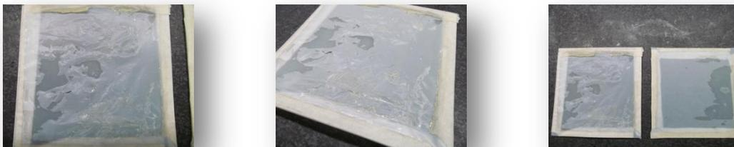
Figure XVIII: Damaged Bath Bottom
