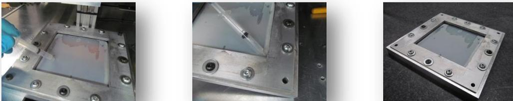
Figure XVI: Removing Photopolymer
