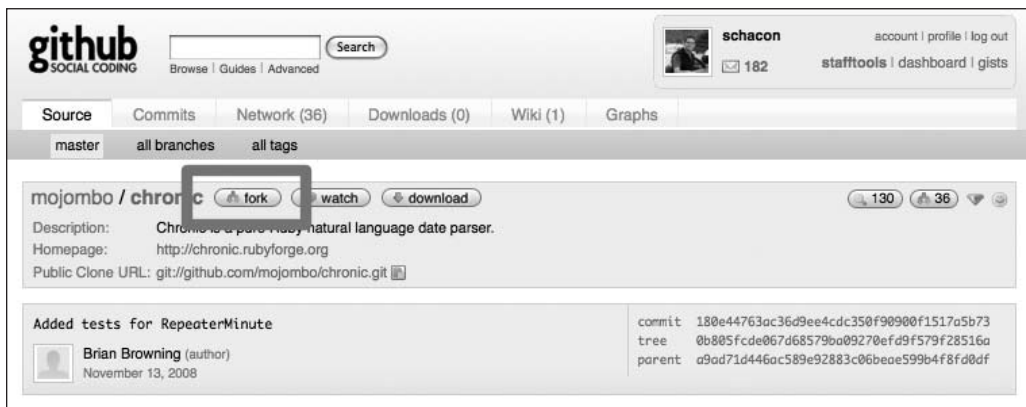
Figure 4-14. Get a writable copy of any repository by clicking the “fork” button.
