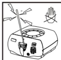
Do not put electrically conductive articles in the machine.
