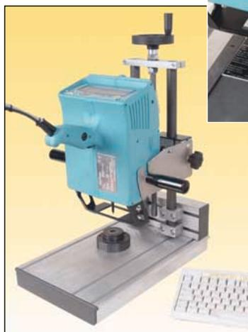
Column frame for marking small parts
