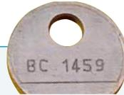
The principle of micro-percussion marking is based on making indents in the material using a vibrating tool. The marking can be carried out on all types of material up to a hardness of 62 HRC: treated or untreated metals, plastics, wood etc... The single marking tool creates permanent markings that are aesthetic and indelible. Due to its design, the marking tool creates low stress in the materials and can mark parts or tags whatever their thickness (from 0.5mm).
