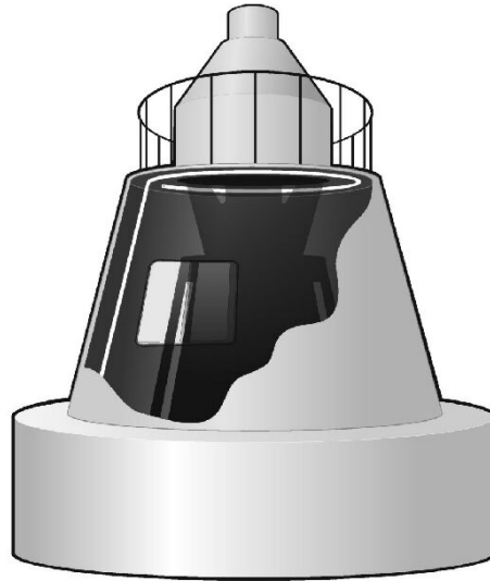
Figure 3 – VESDA sampling pipe curved around the Armature/Commutator housing
