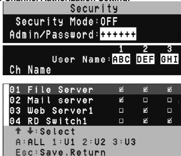
Figure 7-9 PC Channel Authorization Setup
