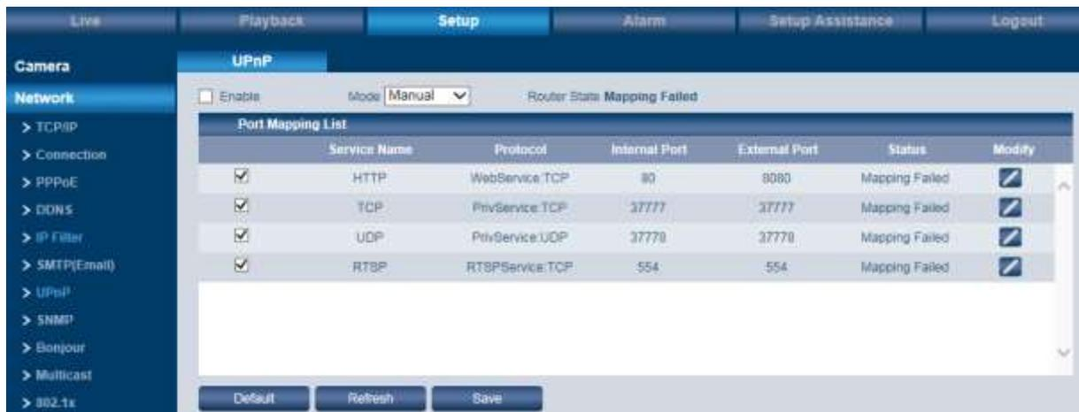
Use UPnP to remotely access your system. In order to use UPnP it is necessary to set Port-Forwarding in your router. You can then access your device using the external address of your router (forwarded port).
