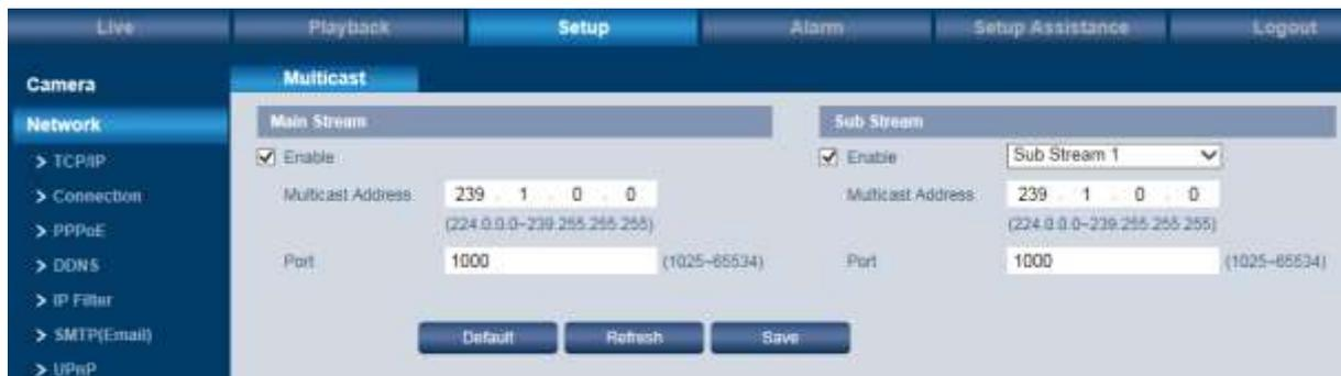
Multicast describes the transmission of data from one point to a group (multi-point connection). When there are multiple hosts to receive the same data packet, multiple cast is the best option to reduce the broad width and the CPU load. Hence data packets can efficiently be sent to several recipients at the same time. This is done by using special multicast IP addresses.
